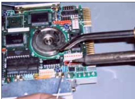
Direct suction at the soldering gun
